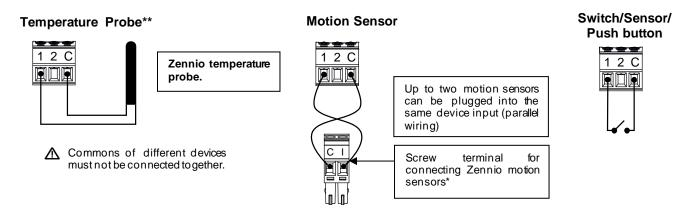
\* In case of using ZN1IO-DETEC-P sensor, its micro switch number 2 must be in Type B position.
