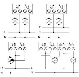
Figure 2: Wiring example (from left to right, and up to down): 2 loads, 2 loads connected to different phases, shutter and fan coil
