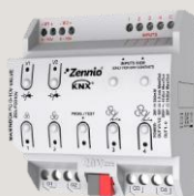
MAXinBOX FC 0-10V FAN (Ref. ZCL-FC010F) Fan coil controller for up to two 2-pipe or 4-pipe units with 0-10 VDC fan speed control signal.*
